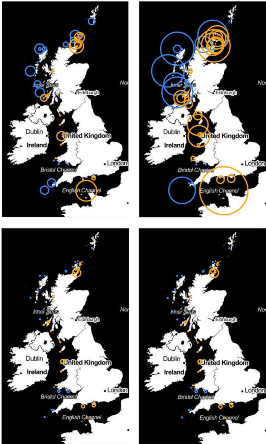
Figure 2. Visual comparison of the installed capacities of wave power (blue) and tidal stream (orange) between 'Low Marine' (top left), 'High Marine' (top right), CT (bottom left), LW (bottom right). There is only a very slight difference between CT and LW. Installed capacity is indicated by the area of the bubble.
