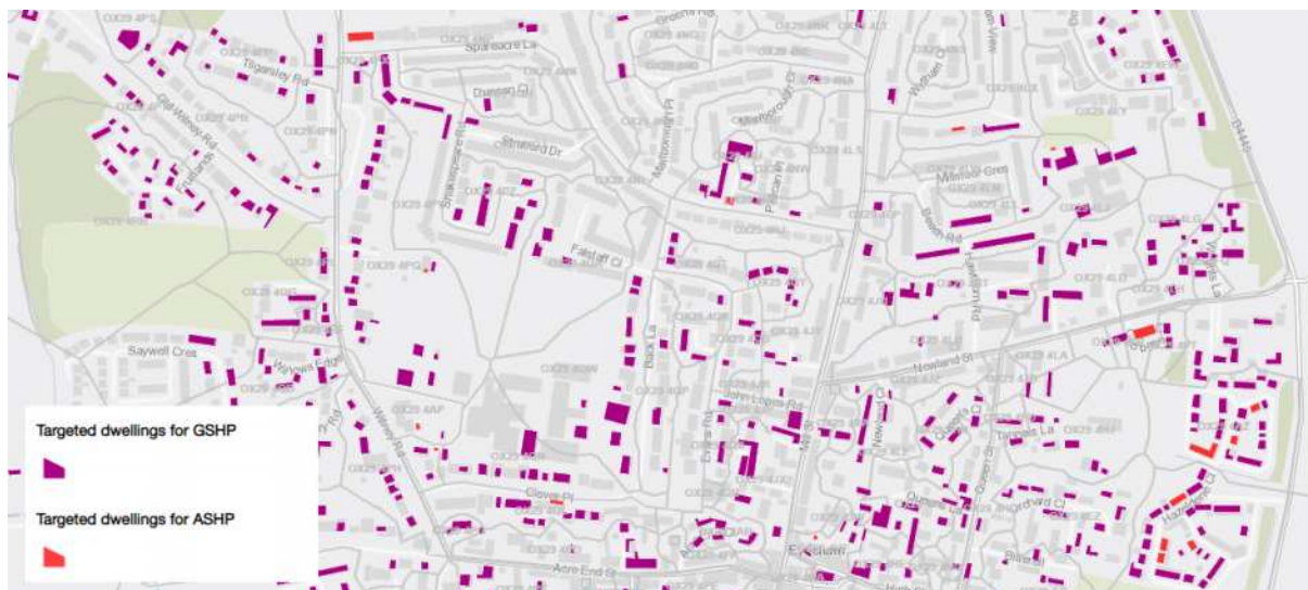
Figure 4. Eynsham Village heat pump suitability
