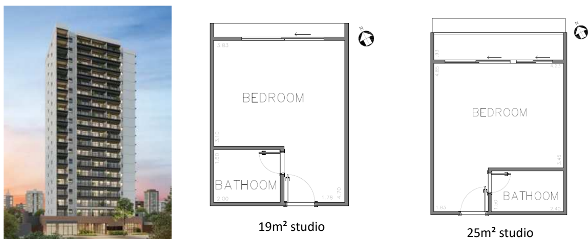
Figure 3. Vila Buarque building facade, and chosen studio apartments' with 19m 2 and 25m 2 (MAC, 2021)
