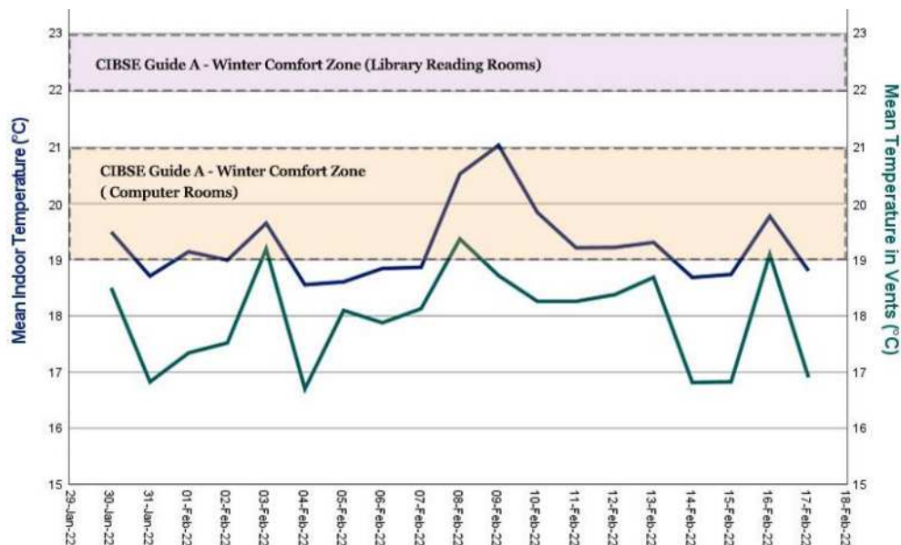
Figure 6. Mean indoor temperature and temperature in vents
